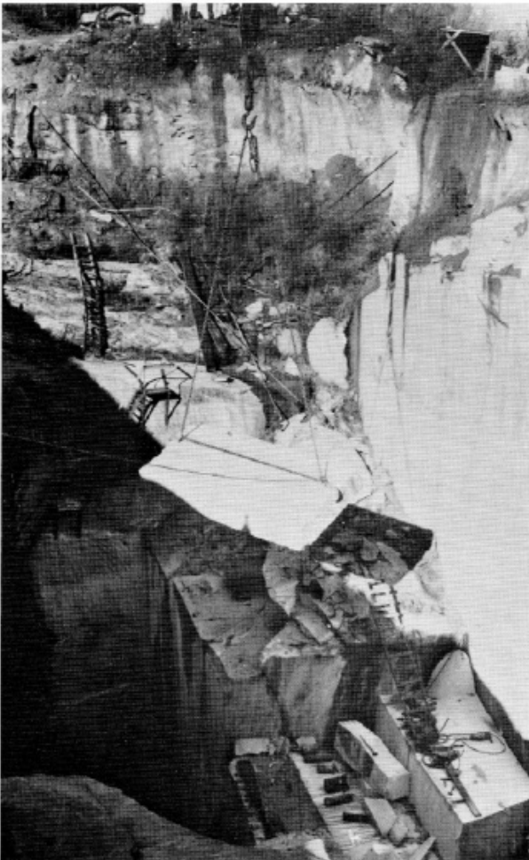
Quarrying was the most crucial phase of The Georgia Guidestones production because of the massive size of the granite slabs and the strain on men and equipment. It was accomplished in the more than 100-ft. depths of the "Pyramid Blue Granite" Quarry. "Our Quarry Superintendent, Jimmy Mattox, and his crew simply did a fantastic job under the circumstances," said Joe Fendley, builder of The Georgia Guidestones .
