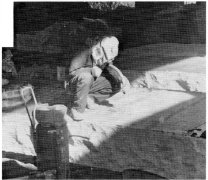
Charlie Clamp, sandblaster on The Georgia Guidestones , is shown etching the "message" into one of the granite slabs. He spent hundreds of hours on the project, which he considers to be one of his greatest undertakings.
