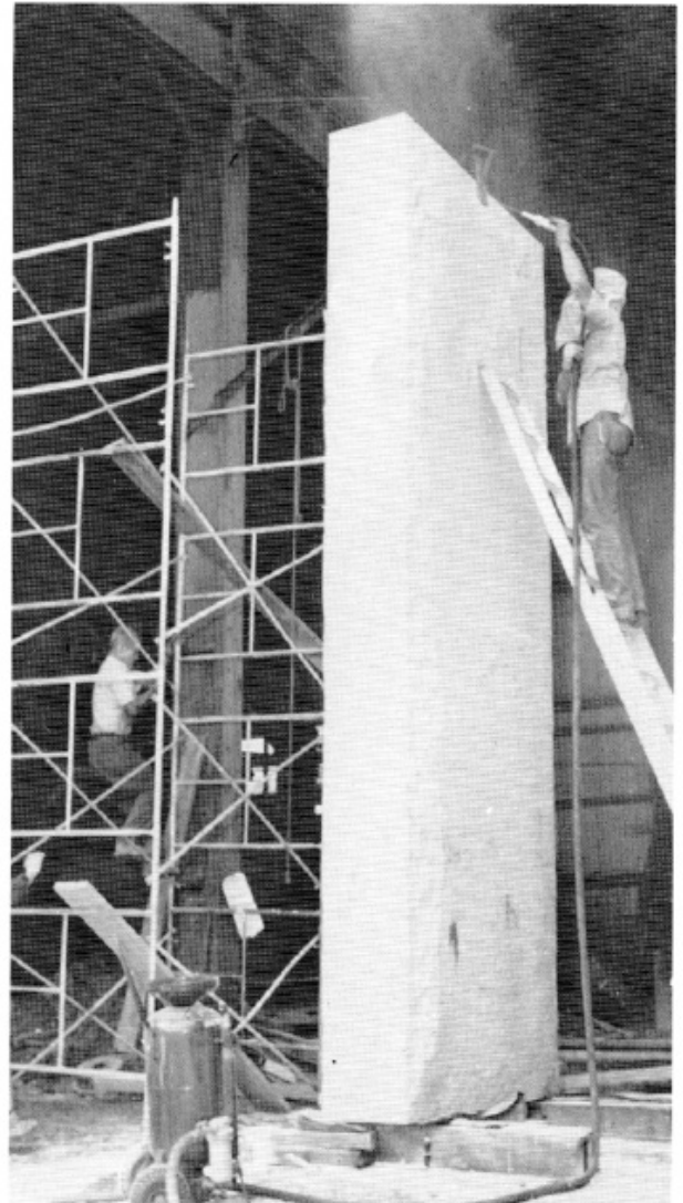
Special scaffolding had to be erected where The Georgia Guidestones® were fabricated so that Charles Clamp could sandblast-inscribe over 4,000 letters which were approximately four-inches high on each stone. The languages were chosen because they represent those spoken by a majority of the people in the world.
